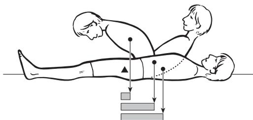
Fig. 1 Movement of the centre of gravity of the upper body during a sit-up exercise.
